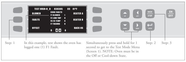
FIGURE 28: Viewing the Fault Log
